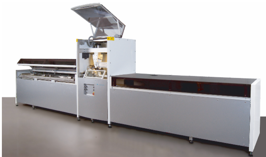
Fig. 1. Front view of the ITRAX core scanner with open hoods. Split core sections are moved incrementally from the left extension to the right extension during analysis.
